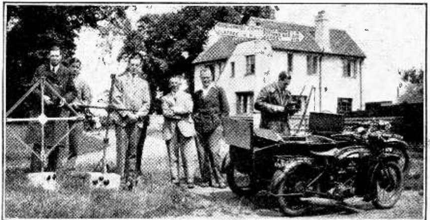
NEW D.F. TEST. The more usual procedure of tracking a concealed transmitter is reversed by the North Middlesex Radio Society recently, when parties with direction-finders, seen above, made unsuccessful attempts to get out of range of a 5-watt transmitter near Ridge, Herts. Two of the receivers shown follow the design of those described by Mr. R. L. Smith-Rose in our issues of August 15th and 29th, 1928.
