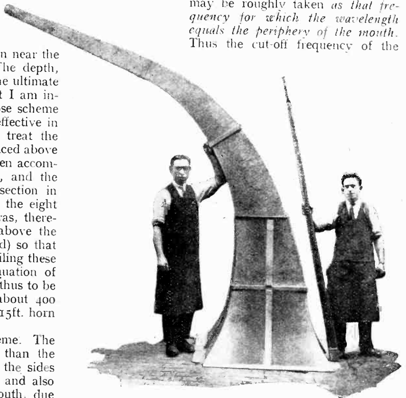
Fig. 2.—Metal portions of experimental 25ft. horn showing on the right the initial straight section which is 8ft. in length.
